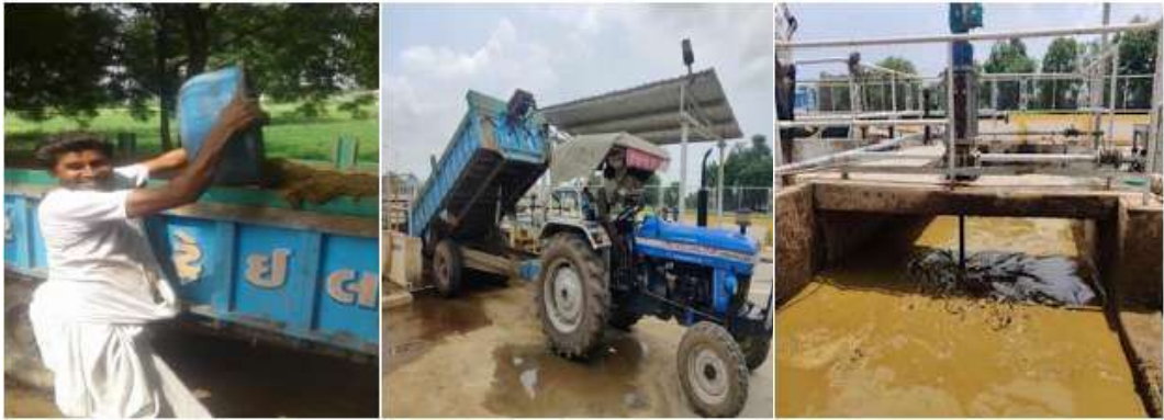
Fig.10: Dung Loading, Unloading and Mixing with Water
