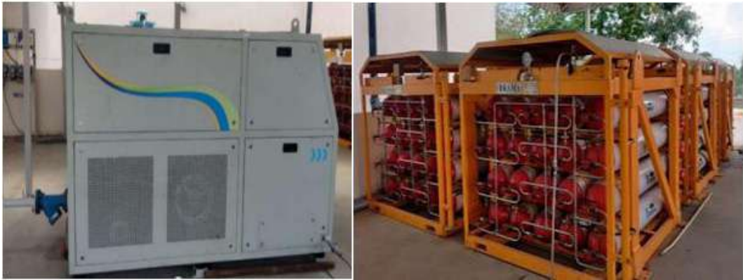
Fig.14: Biogas Compression and Bottling Unit
