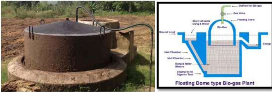
Fig.7: Floating Dome Biogas Plant and Its Schematic View
