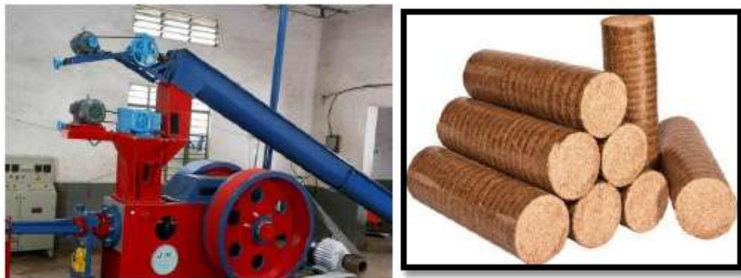
Fig.6: Biomass Briquetting Machine and Briquettes
